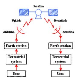
Figure 1. Block diagram of satellite communication
